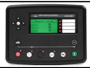
The DSE8610 is an easy to use multi-generator loadshare system, designed to synchronise up to 32 generators including electronic and non-electronic engines. The DSE8610 monitors the generator and indicates operational status and fault conditions, automatically starting or stopping the engine on load demand or fault condition.
