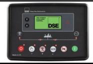
The DSE6120 is an Auto Mains (Utility) Failure Control Module suitable for a wide variety of single genset applications. Monitoring engine speed, oil pressure, coolant temperature, frequency, voltage, current, power and fuel level, the modules will give comprehensive engine and alternator protection.
