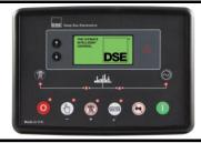
The DSE6020 is an Auto Mains (Utility) Failure Control Module suitable for a wide variety of single genset applications. Monitoring engine speed, oil pressure, coolant temperature, frequency, voltage, current, power and fuel level, the modules will give comprehensive engine and alternator protection.
